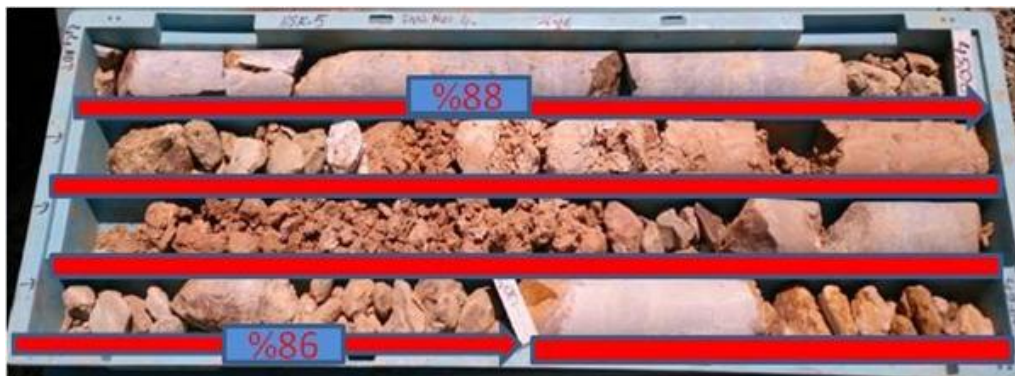
Figure 4. View of the cores obtained from the HSK-5 borehole.
